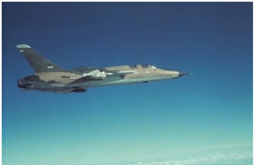
This F-105F is the one flown by Thorsness on his memorable mission. It was specially configured to defeat enemy missiles with radar and missile-launch warning systems and radar-seeking Shrike missiles.
